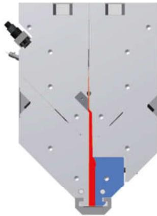
For customer who need greater lip gap range, ( $>\pm 2\text{mm}$ ), the replaceable die lip system can be implemented. Lip gap adjustment range can reach  $50\text{mm}$  when the lower lip is replaced. (Production needs to stop for replacement)
