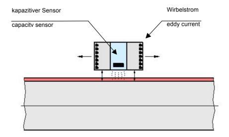
indirect measurement (measurement of sheet property – calculation of thickness) capacitive sensor: measurement of property (capacity: depending on dielectric) eddy current sensor: measurement of distance (sensor – roller)
