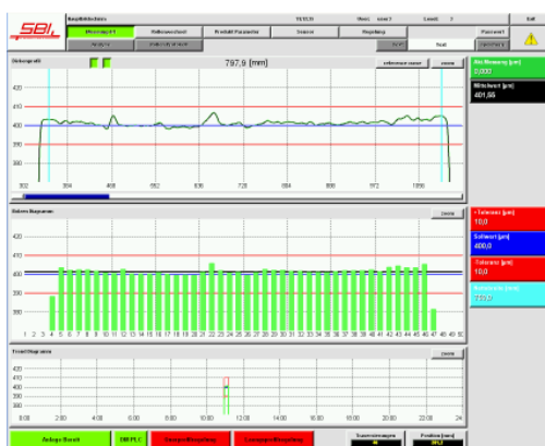
Main screen: thickness- and bolts diagram
