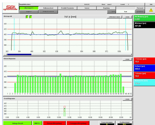
Main screen: thickness- and bolts diagram
