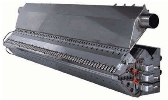
Thermal bolts utilizes thermal expansion of steel bolts
