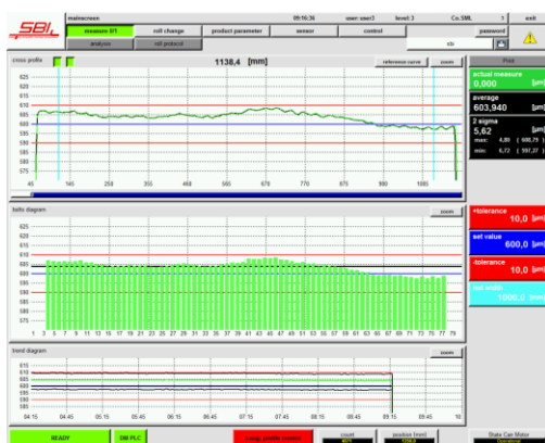
Main screen: thickness- and bolts diagram
